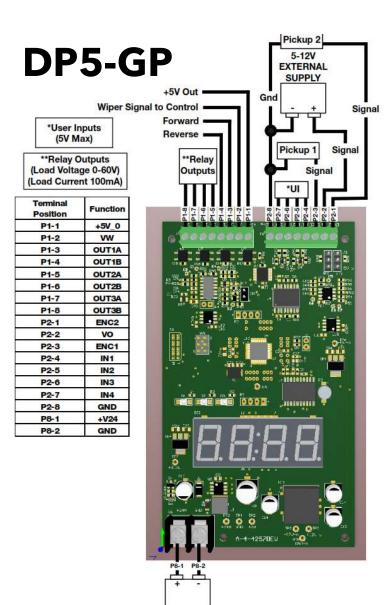
The Dart DP5 can be so much more than just a Digital Potentiometer. There are four each digital User Inputs (UI) and digital Relay Outputs. This creates the opportunity for the DP5 to execute logic, timing and sequencing scenarios, potentially eliminating other components in the OEM panel.
